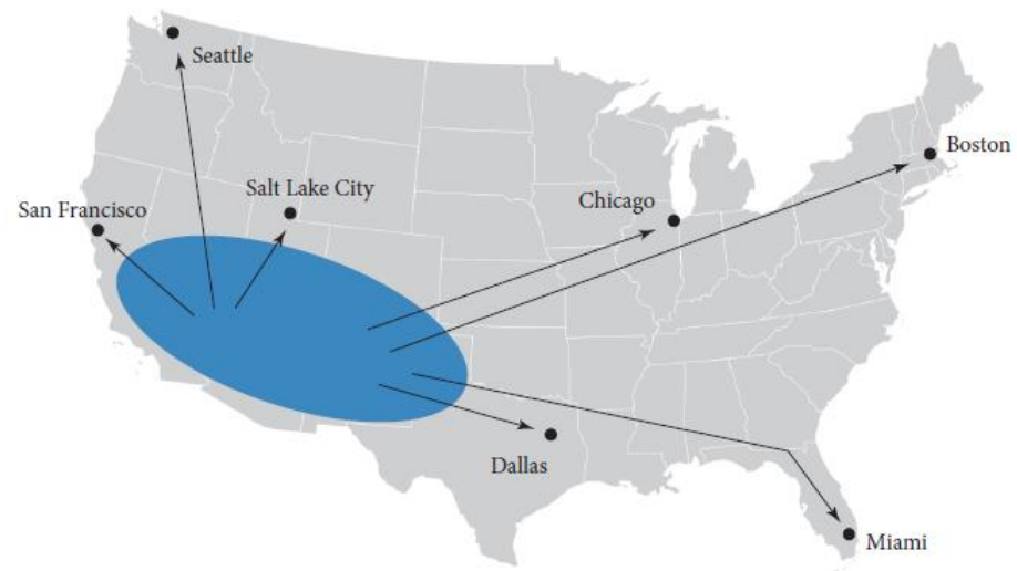
Fig. 10.4 Possible HVDC grid for transmitting solar energy across the USA. Source: DOE2007.
